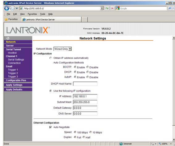
**6** Select the "IP Address" item in the "IP Configuration", and enter the correct address value.
