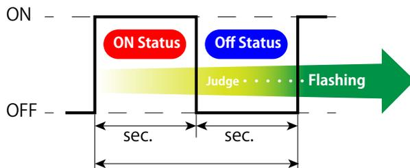
ON + OFF for one cycle=Flashing
