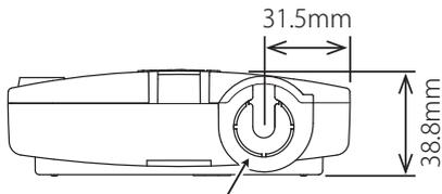
Cable Gland Mounting Hole (Break-out)
