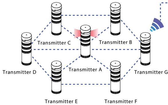
Multi-hop network communication is flexible enough to change in response to radio communication circumstances. The transmitted data mutually selects the best route for radio wave communication. Even with modifications of the floor layout, data communication starts automatically from power-up.
